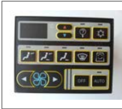
KLİMA KONTROL PANELİ Air Conditioner Control Panel
